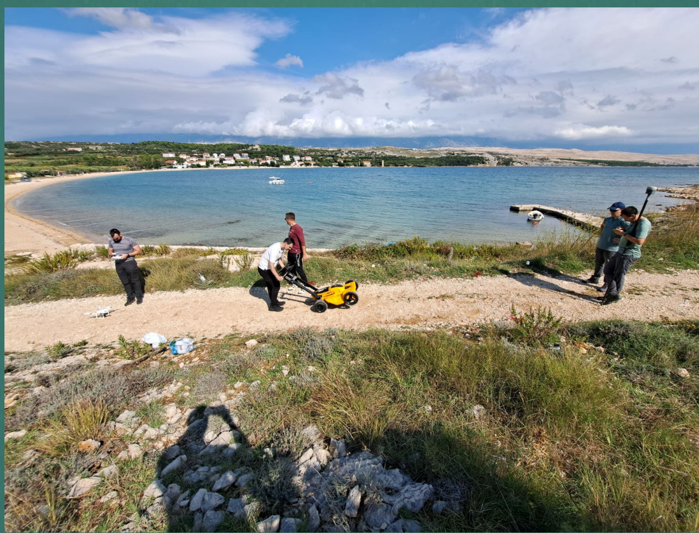
Fig 2. Georadar survey in Caska Bay
